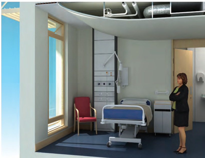
Figure 2: A design solution to overcome building codes that restrict window openings to 100mm: there is a 100mm opening at low level and then a larger opening at high level, where the ceiling has been cut away to give maximum height. This system is in use at Altnagelvin Hospital, Northern Ireland
